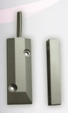
Brand e-5continents Certificate: CE (5CPS-55) Dimension 106\*38\*10mm (switch) 106\*16\*16mm(magnet) Housing Metal(Alloy-Zn ), grey Gap 50-70mm 60-70mm available Output N.C. N.O. & Changeover available Leads 1007UL22AWG530mm, with 380mm stainless steel cable Package Inner packing 1set/PE, each part packed individually Outer packing 50sets/carton Gross Weight 60.0KG Remarks 4 screws including
