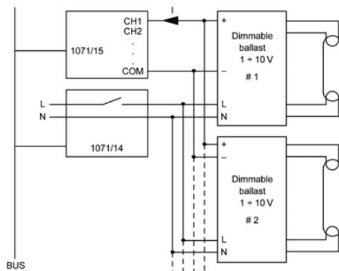
In both cases, a linear or logarithmic type output ramp can be defined.
